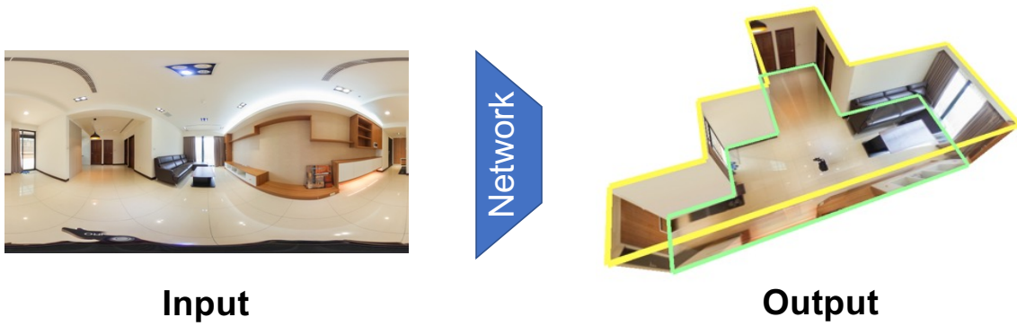
Figure 3.1: The task for layout estimation [3]. Given a single panorama, we train a neural network that takes the panorama as input and infers the corresponding 3D structure.
