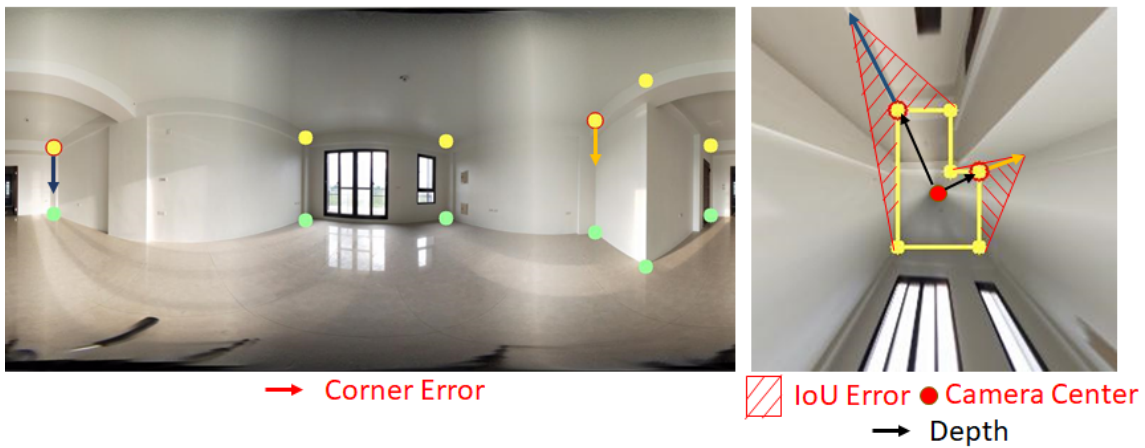
Figure 3.2: The motivations of LED 2 -Net [3]. The corners of a room layout are shown in the left figure. When we introduce same errors to these corners, the IoU difference introduced from these corner errors can be hugely different (right figure).
